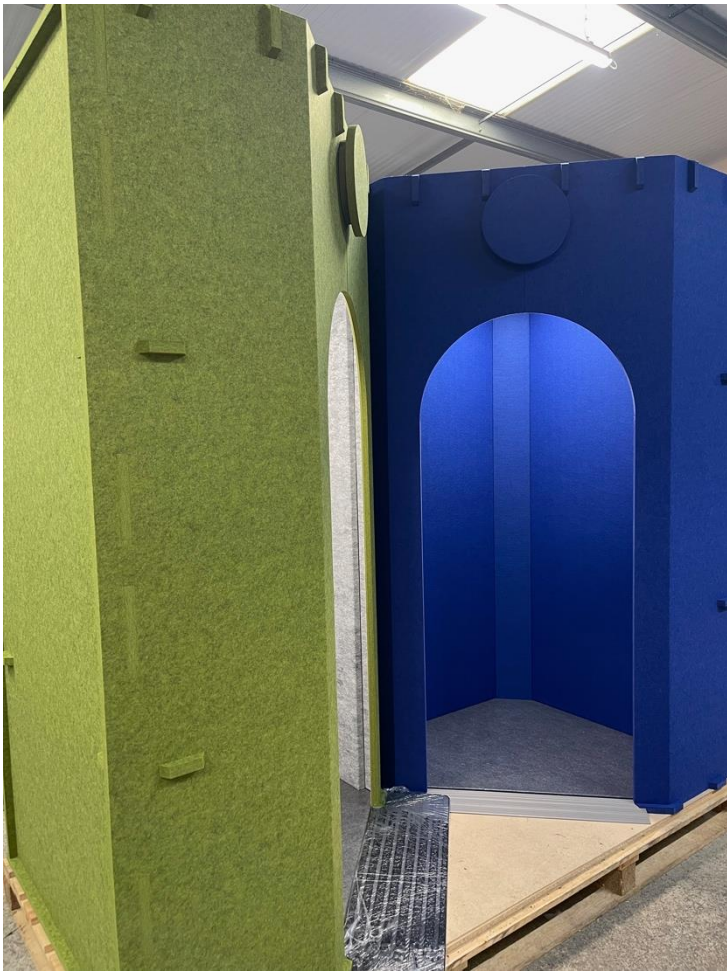
Corner Pod tested in factory with background noise, then showing reduction when entering the Pod.
